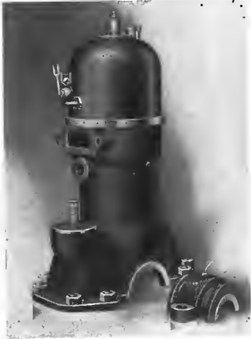
Cylinder Casting, Showing Intake Valve.
